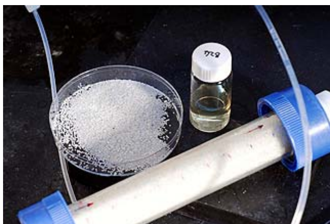
Laboratory equipment used to study the transport and retention of C 60 nanoparticles in water.
