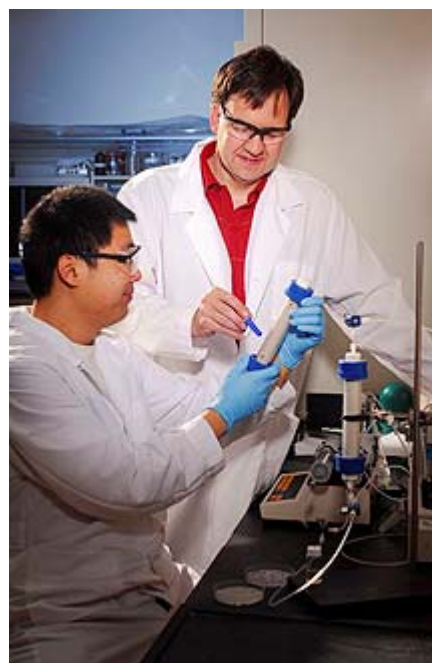
Researchers Kurt Pennell (standing) and Younggang Wang examine glass columns used to measure the transport and retention of C 60 particles in water.
