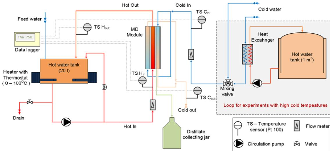
Fig. 3. Sketch of laboratory scale experimental setup
