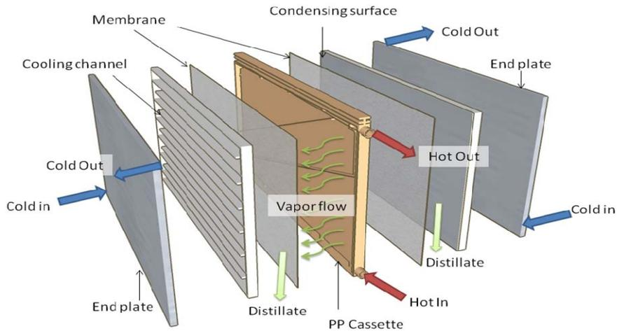
Fig. 1. Sketch of a Laboratory scale MD module
