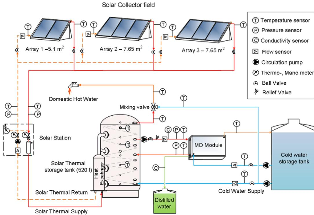
Fig. 5. Sketch of pilot experimental setup of SDHW-MD system
