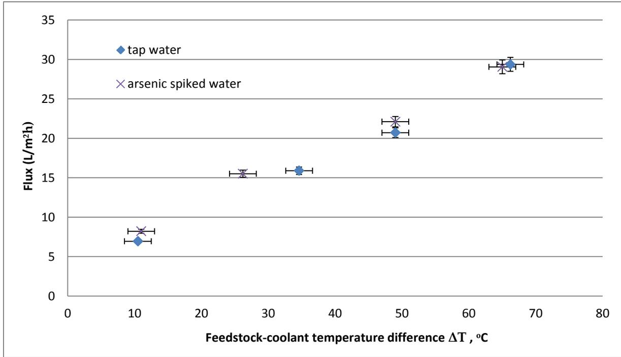
Fig. 2 - Product water flux as a function of temperature difference across the membrane (feed water flow 3.8 L/min, coolant flow 1.9 L/min, feedwater inlet temperature ca 80°C, coolant inlet temperature varying)
