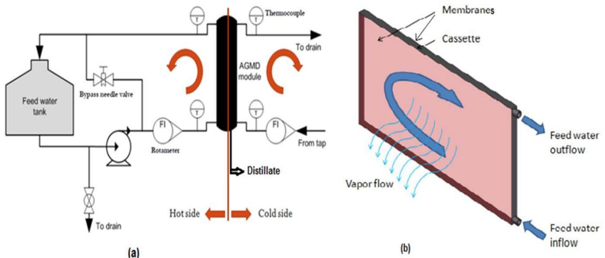
Fig. 1 - (a) MD bench scale unit setup at KTH (b) Membrane Cassette (MD)
