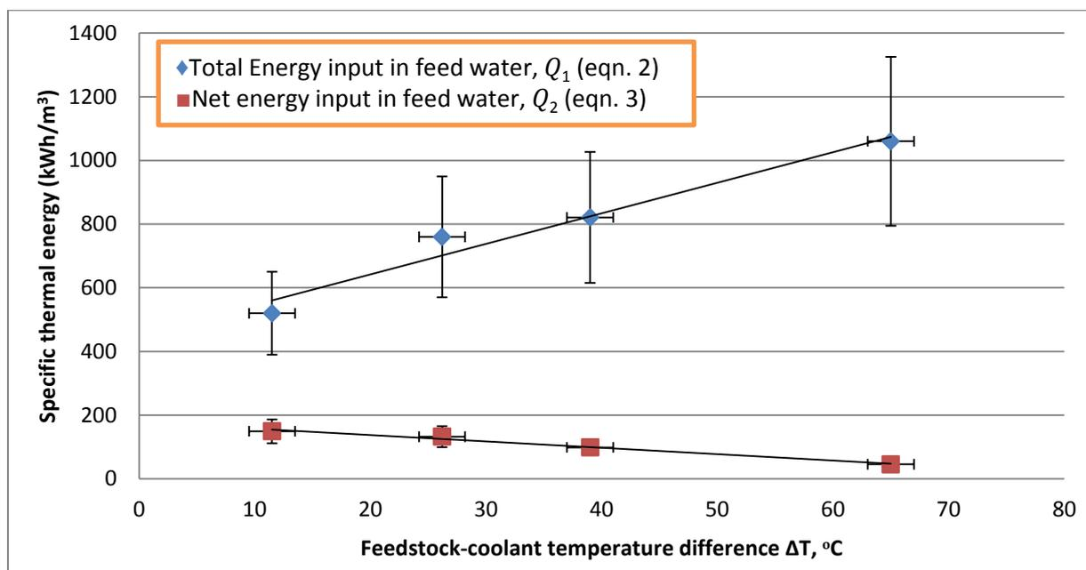
Fig. 3 - Specific thermal energy consumption for AGMD module (feed water flow 3.8 L/min, coolant flow 1.9 L/min, feedwater temperature ca 80°C, coolant temperature varying)
